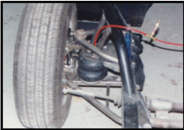
Aftermarket Mustang II installation [replaces coilover shock]
