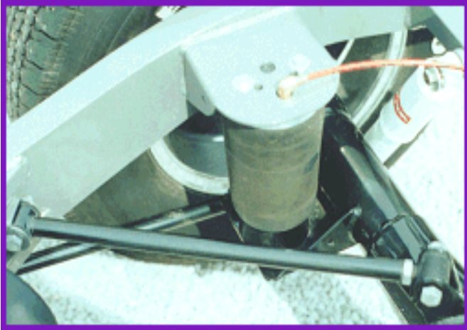
Rear suspension w/ 4 link and air ride
