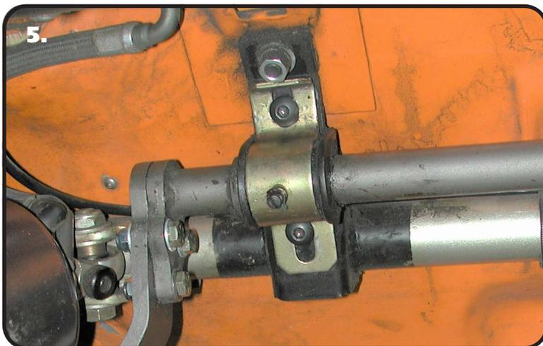
5. Bolt the sway bar to the AirBar bridge. Use 3/8" x 1" button heads on the front and 3/8" x 1/2" button heads on the rear mounting holes with lock washers. Torque to 16 ft-lbs
