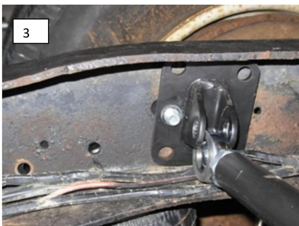
3. On the truck we done a preexisting hole captured the middle hole(fig3) in panhard bracket. This bracket can be welded or bolted to the frame using the supplied 1/2" hardware. Insert the R-Joint Spacers and bolt the bar to the bracket using 5/8" x 3" bolt, flat washers, & 5/8" nylok nut.
