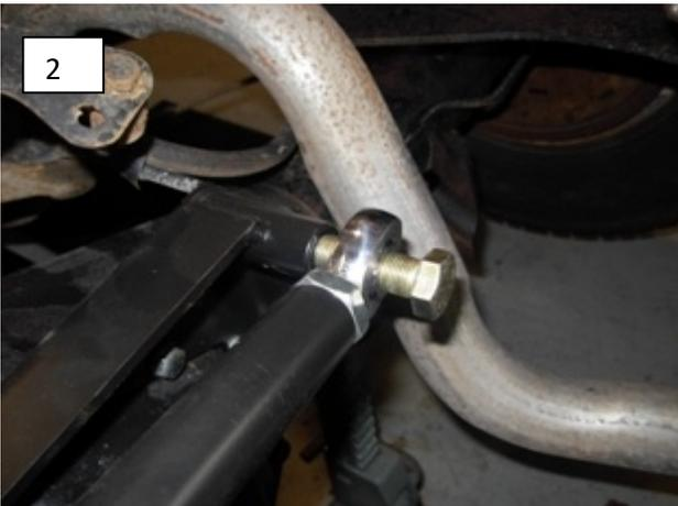
2. (fig2) Use the panhard bar as a guide to locate the panhard frame mount. The Panhard bar should be level at ride height. The bar gets bolted to the bracket using a 5/8" x 3" bolt, flat washer, and a split lock washer.
