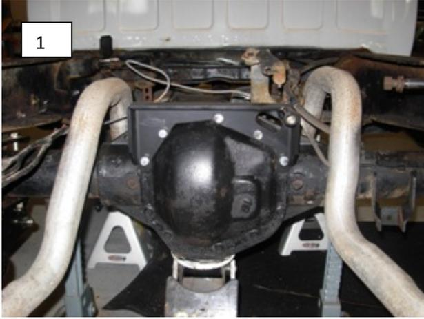
**Insert the Spacers into each side of the R-joint.**
