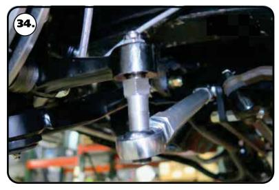
**34.** Install the outer end of the tie rod on the steering arm stud.
