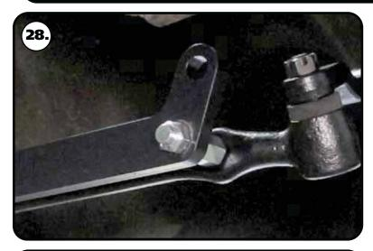
**28.** Install the 1/2"-20 mechanical locking nuts and torque to 50 ftlbs.
