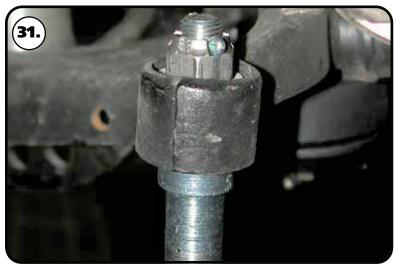
**31.** Install the stud with the round flange into the steering arm with the taper going into the steering arm. Torque the nuts to 35 ftlbs and tighten as needed to align cotter pin hole and install cotter pin.
