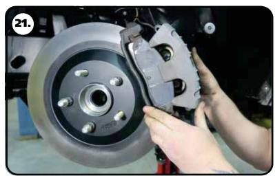
**21.** Install the brake pads and caliper.
