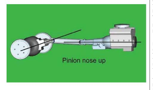
12. How do you set the pinion angle? On a single-piece shaft you want to set it up where a line drawn through the center of the engine crankshaft or output shaft of the transmission and a line drawn through the center of the pinion are parallel to each other but not the same line.
