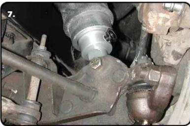
The air fitting location can be rotated by twisting the bellow assembly separate of the shock. Place the Shockwave into the OEM shock location with the stud sticking through the OEM shock hole. See assembly Diagram
