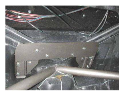
6. The inner support plate will bolt to the floor pan on the inside of the car using six  $3/8^{\circ}$  x 1" bolts, Nyloks and flat washers. The remaining 4 holes will need to be drill and will use  $3/8^{\circ}$  x 2  $\frac{1}{4}^{\circ}$  bolts, Nyloks and flat washers.
