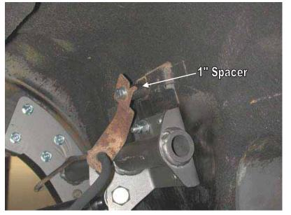
17. Insert a 5/8" x 4" bolt through the upper mount and Shockwave eye. There should be a 5/8" flat washer on each side of the poly bushing and one next to the head of the bolt. Fasten the assembly with a 5/8" Nyloc nut.
