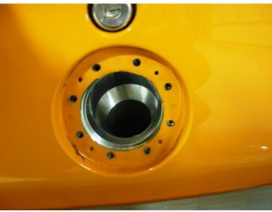
5. Remove the cap and drill the holes with a 3/16" bit.
