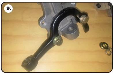
9. We suggest using RED Threadlocker on the steering arm mounting hardware. Line up the steering arm mounting holes with the bottom 2 holes of the spindle. Insert the 2" long bolt through the thick boss and the 1 3/4" long bolt through the thin boss, threading the bolts into the spindle. The steering arm hardware will need to be torqued to 100 ftlbs, but it is easier to torque with the spindle installed on the car.
