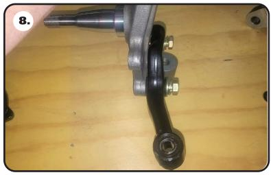
**8.** The steering arm will bolt to the BOTTOM set of holes in the Ridetech spindle using the supplied 1/2" hardware. The mounting bosses of the steering arm are 2 different thicknesses. The thicker boss uses a 1/2"-20 x 2" hex bolt. The thin boss will use a 1/2"-20 x 1 3/4" bolt. Install a 1/2" split lock washer followed by a 1/2" SAF flat washer on each bolt.
