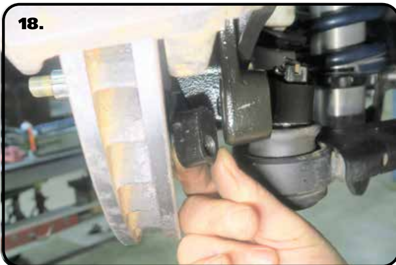
18. Insert the steering arm inserts into the spindle using the correct orientation from the details above.
