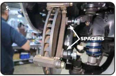
**5.** The kit includes spacers that will be installed between the caliper bracket and caliper mount. Install a M14 flat washer on each of (2) M14-2.0 x 45mm hex bolts. Insert the bolts through the caliper bracket, installing a spacer on each bolt. Line the caliper mount up with the hardware and thread in the bolts.
