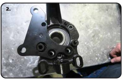
**2.** The caliper brackets are side specific. They have a D & P stamped in them. Lay the correct side caliper bracket on top of the shims, aligning the mounting holes with the mounting holes of the bracket. The counter sunk holes should facing up.
