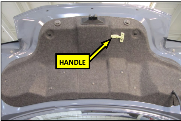
1. Raise the trunk lid and remove the emergency release handle from the trunk lid liner.
