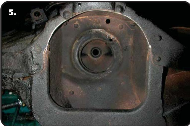
5. For air spring clearance some trimming must be done around the coil spring pocket. This is what it should look like after cutting. This is best done with a cut off wheel or plasma cutter. Grind all cuts smooth when finished.
