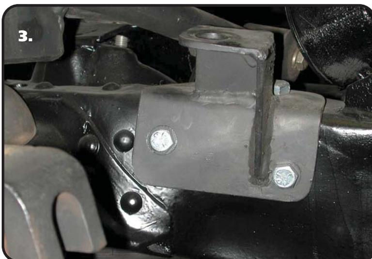
3. Place the upper shock mount on the corner of the frame behind the upper control arm. Slide it forward until it touches the rivet as shown the picture. This is the driver side. Use the bracket as a template to mark and drill the two holes on top of the frame. Secure the bracket with 7/16" x 1" bolts, nylok nuts, and washers. Then drill and bolt the one closest to the rivet, and finish up on the rear hole. Torque to 50 ft-lbs.
