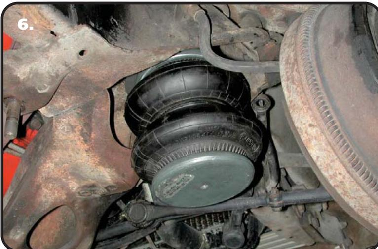
6. Install air spring assembly into the coil spring pocket with the tall side of the bracket towards the wheel. With the stud protruding through the OEM shock hole. (The airline must also be routed at this time.)
