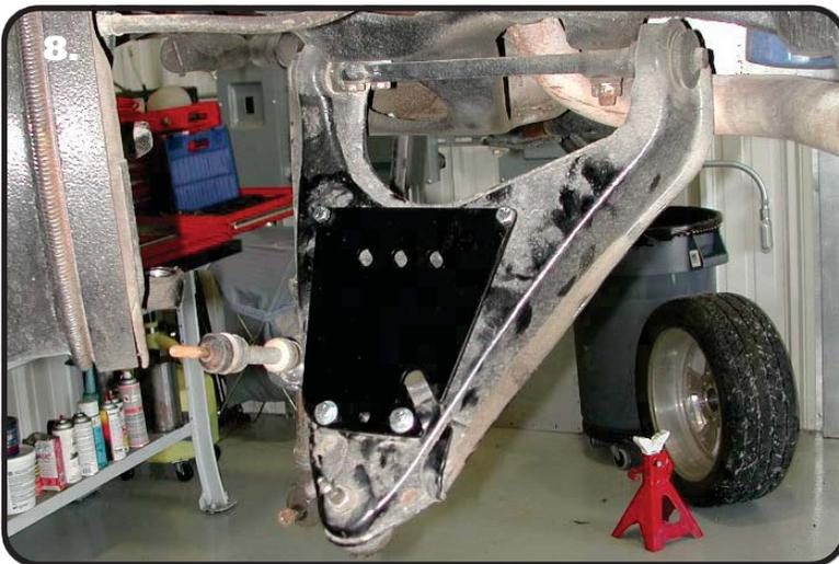
8. Bolt the lower air spring plate to the lower arm. The two outer holes will align with the factory bump stop holes. The inner two holes must be drilled. Use the bumpstop to bolt the outer part of the plate to the control arm. Use a 3/8" drill bit to drill the inner 2 holes. Instal a 3/8" flat washer on each of (2) 3/8"-16 bolts and insert them into the holes. Install a 3/8" flat washer and 3/8"-16 nylok nut on the threads of the bolt. Torque to 30 ft-lbs.
