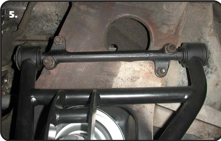
5. The Lower Control Arm is attaching the frame using factory hardware. The driver side arm is shown in **Figure "3"**. Torque the hardware 65-75 ft-lbs.
