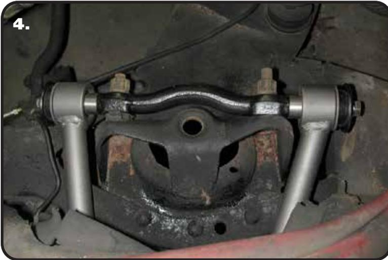
4. The Upper Control Arm is attaching the factory mount using factory hardware. Reinstall the shims in the location they were removed from. The passenger side arm is shown in **Figure "4"**. Torque the hardware 65-75 ft-lbs.
