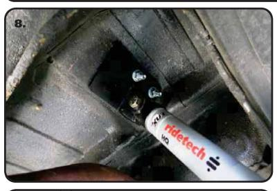
**8.** The Shock is mounted in the Upper Mount with the BODY UP. It is held in place with a 1/2"-13 x 2 1/2" Hex Bolt & 1/2"-13 Nylok with a 1/2" Flatwasher on each side of the bracket.
