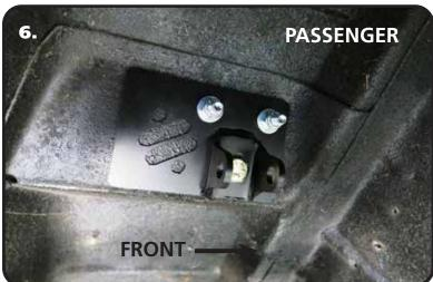
**6.** The Passenger upper Shock Mount keeps the shock in the OEM location, but converts the shock to an eyelet. There's 3 holes in the bracket for mounting, (2) 7/16" & (1) 1/2". The 1/2" hole uses the OEM shock hole as a locator. Insert a 7/16"-14 x 1 1/2" bolt into the 1/2" hole. Position the mount with the 7/16" bolt inserted into the OEM shock hole. Align the inside edge of the mount with the body. Mark and drill the 2 remaining holes with a 3/8" drill bit.
