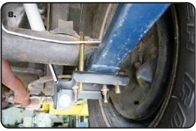
**8.** Lower the differential onto the Leaf Spring. Align the top PIN into the HOLE in the OEM leaf spring mount. Install the lower Clamping Plate/Shock Mount, supplied in the Staggered Shock Kit being sure the Pins and Holes are aligned. The Clamping Plates have the shock mounts built in, the driver mount is installed with the shock mount to the inside rear with the passenger installed with the shock mount to the inside front. Driver is shown in Diagram "6". Install the 7/16" U-Bolts.
