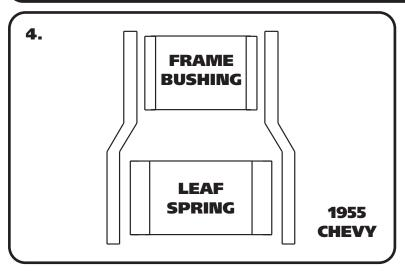
**4.** The orientation of the Shackle Plates is determined by the year of the car. The Frame bushing is 2 1/2" wide on a 1955, 3 1/2" wide on 1956-1957. 1955 is shown in Diagram "6". The 1955 uses 1/2"-13 x 4" in the FRAME bushing and 1/2"-13 x 4 1/2" in the REAR leaf spring bushing.
