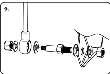
**9.** The Lower Shock is Bolted to the Lower Shock Mount using the supplied Shock Stud. Insert the Shock Stud into Lower Mount with a 5/8" Flat Washer on EACH side of the mount. Install a 5/8" Lock Nut on the threads and tighten. Next, slide a Washer on the Shock Stud. Jack the Rear Differential up until the Shocks can be slid onto the Shock Studs. Install a 7/16" Flat Washer and 7/16" Hex Nut onto the Threads and tighten.
