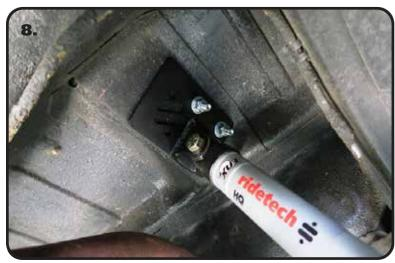
**8.** The Shock is mounted in the Upper Mount with the BODY UP. It is held in place with a 1/2"-13 x 2 1/2" Hex Bolt & 1/2"-13 Nylok with a 1/2" Flatwasher on each side of the bracket.
