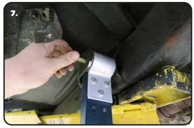
7. Bolt the **NARROW BUSHING END** of the Composite Leaf Spring into the OEM front leaf spring mount using a 1/2"-13 x 4" Hex Bolt and 1/2"-13 Nylok Nut.
