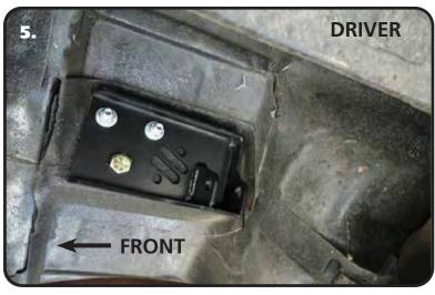
**5.** The Driver upper Shock Mount repositions the top of the shock. There are 3 holes in the bracket for mounting, (2) 7/16" & (1) 1/2". The 1/2" hole uses the OEM shock hole as a locator. Insert a 7/16"-14 x 1 1/2" bolt into the 1/2" hole. Position the mount with the 7/16" bolt inserted into the OEM shock hole. Align the inside edge of the mount with the body. Mark and drill the 2 remaining holes with a 3/8" drill bit.
