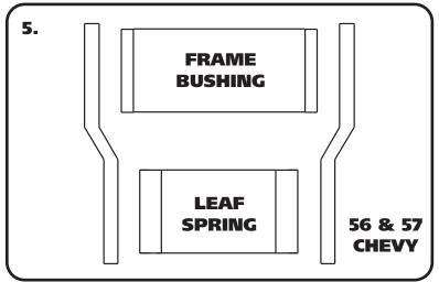
**5.** Diagram "5" shows the Shackle Plate orientation for 1956 & 1957. These cars use 1/2"-13 x 5" in the FRAME bushing and 1/2"-13 x 4 1/2" in the REAR leaf spring.
