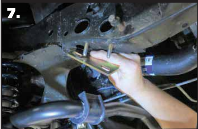
7. Install a 5/16" flat washer on each of (2) 5/16"-18 x 1 1/4" bolts and insert them into the OEM sway bar holes by inserting them in through the access holes in the side of the frame. Install the spacer plate with the wide side positioned to the inside. Hold it in place.
