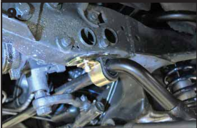
9. Lift the bar in position, the bolts sticking through the frame and spacer will go in the slots of the bushing strap. Hold the bar in place & install a 5/16" flat washer and 5/16"-18 nylok nut on the threads of each bolt sticking through the slots of the bushing strap. Repeat steps 8-10 on the opposite side, but do not tighten the hardware at this time.
