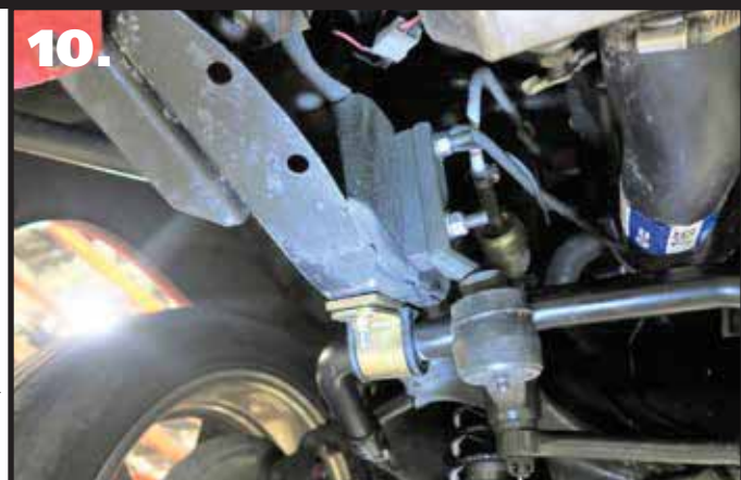
10. Reattach the idler arm to the frame using the OEM hardware. Torque the hardware.
