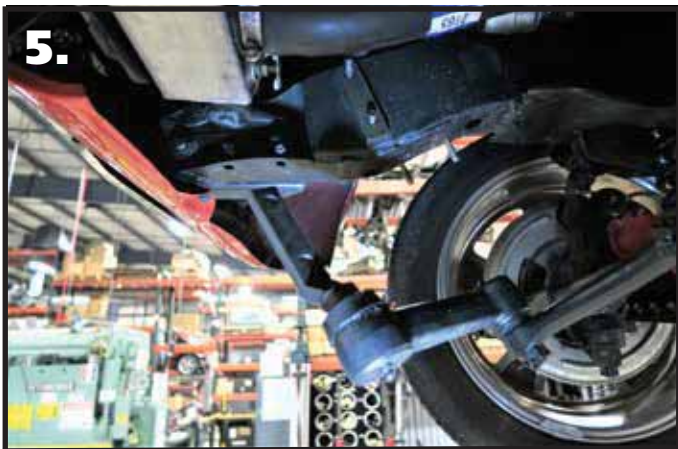
5. Disconnect the idler arms from the frame.
