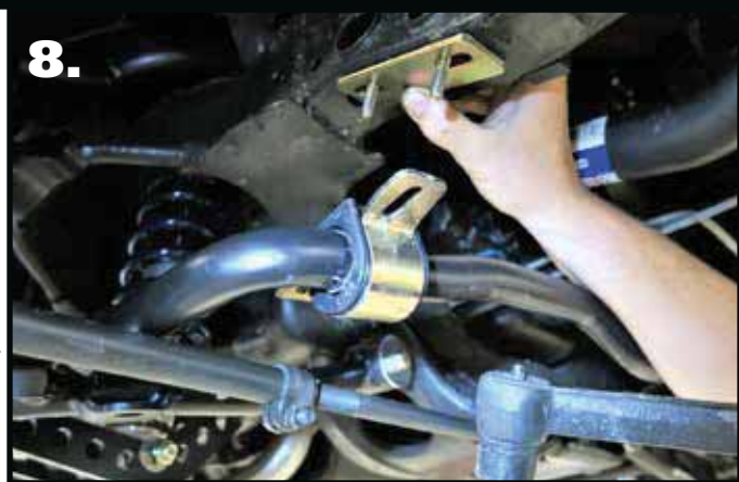
8. Install the bushing strap over the swaybar bushing with the wide side of the strap to the inside on the car. We found some steering box conversions hang down further than others. If yours happens to hit the sway bar, add a 2nd spacer under the bushing. a 2nd set of spacers along with longer hardware is supplied in this kit.
