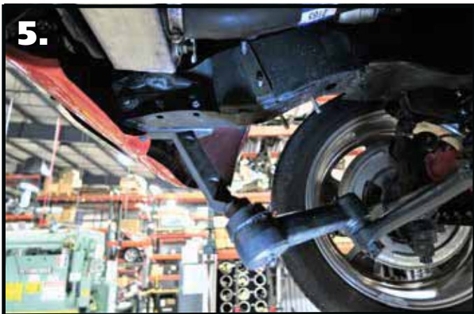
5. Disconnect the idler arms from the frame.
