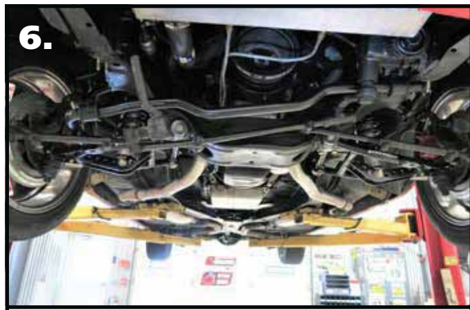
6. Insert the new swaybar from the passenger side. position it above the idler arm and steering arm. the center of the bar should hang down towards the ground.
