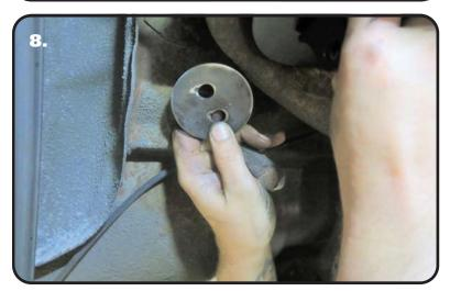
**6.** The Upper Mount is attached to the frame using (2)  $1/2"-13 \times 1 1/2"$  Bolts. Insert the bolts through the shock mount and into the upper plate.
