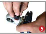
Install upper spring mount retainer clip (803-00-199) into the groove on the upper eyelet as seen in figure 5. Then, reinstall adjuster to complete assembly.
