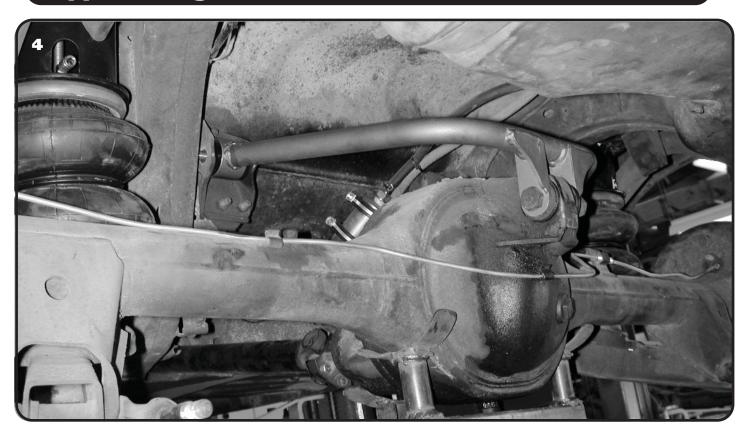
**4.** Bolt the new upper control arm in the OEM location using the hardware supplied in the kit. The control arm is attached to the car using (3)  $1/2"-13 \times 3 1/2"$  bolts, 1/2" flat washers, and 1/2"-13 nylok nuts. Tighten the hardware enough to eliminate any gaps.
