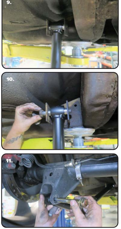
**9.** The Lower Control Arm has the bottom CoilOver mount built in, it will need to be installed with the CoilOver mount up and to the rear of the car. Install a 5/8" ID R-joint Spacer into the front R-joint. The Small Diameter goes into the R-joint. Slide the R-joint into the OEM lower control arm mount. Align the holes in the frame with the thru-hole of the R-Joint.
