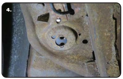
**4.** The frames of these cars varied through the years, some have a center hole, some are solid. The frame we are doing this install on has a center hole. If the frame is solid, drill the marked holes with a 1/2" drill bit. Frames with the center hole will require a die-grinder or something similar to notch the edges of the center hole. We used a die-grinder with a burr bit to notch the holes. Repeat **Steps 2-4** on the opposite side.
