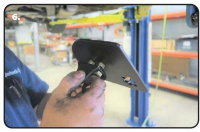
**6.** The Upper Mount is attached to the frame using (2) 1/2"-13 x 1 1/2" Bolts. Insert the bolts through the shock mount and into the upper plate.
