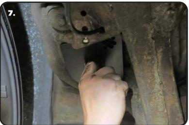
**7.** Position the Shock Mount/Plate up into the frame, holding the shock mount and hardware in place.
