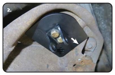
2. This kit contains a Upper Shock Mount setup that will require drilling to install it. Image 2 is of the upper mount installed, we will cover the installation in the next steps. The rear of the plate will need to be aligned with the body mount that is to the rear of the coil spring mount. See the ARROW in Image 2.
