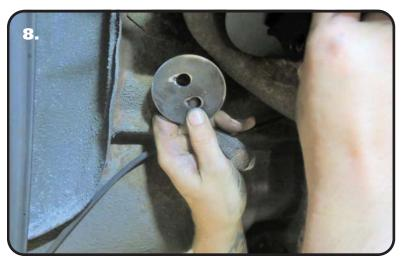
**8.** Install the Upper Backer plate by installing it on the 1/2" bolts that are sticking through the top side of the frame. Install a 1/2"-13 nylok nut on each of the bolts sticking through the frame and backer plate. Torque the hardware to 75 ftlbs. Repeat for the second side of the car.
