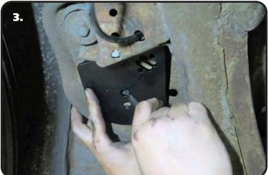
**3.** The upper mount bolts into the car and will require the holes to be drilled. Start by holding the plate up in the car aligning the back edge with the body mount. Mark the holes on the frame.
