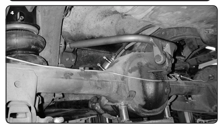
**4.** Bolt the new upper control arm in the OEM location using the hardware supplied in the kit. The control arm is attached to the car using (3)  $1/2"-13 \times 3 \cdot 1/2"$  bolts, 1/2" flat washers, and 1/2"-13 nylok nuts. Tighten the hardware enough to eliminate any gaps.
