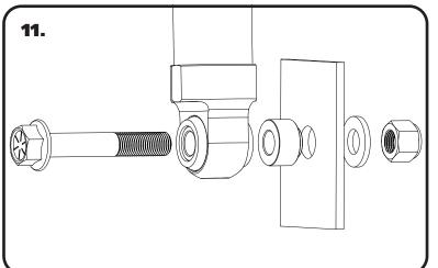
**11.** Insert the  $\frac{1}{2}$ "-20 x 3" flanged head shock bolt through the lower shock eye and then place the aluminum spacer onto the stud. The step on the spacer will go into the arm. Slide the stud through the tab on the lower arm and secure w/ nut and washer. Torque to 75 ft-lbs.
