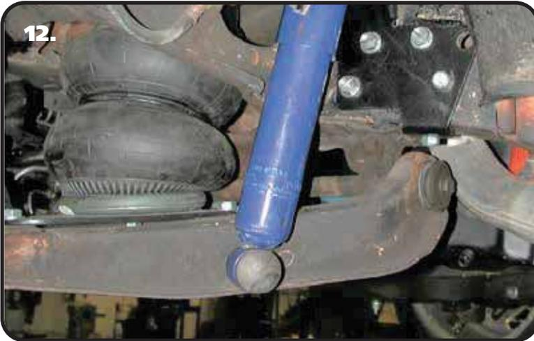
12. Drill a 5/8" hole in the lower control arm approximately 7 3/4" from the cross shaft bolt.
