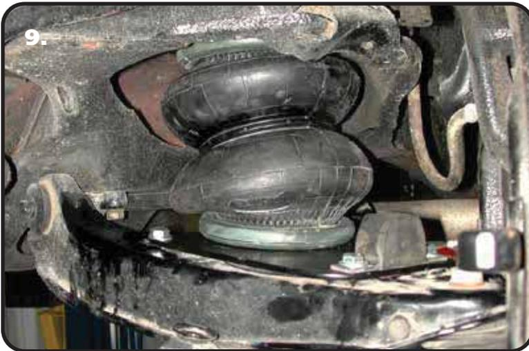
**9.** The air spring will be attached to the lower plate using a 3/8" x 3/4" bolt, lock washer and flat washer. It will get bolted to the middle of the 3 holes. Torque the 3/8" bolt 15-20 ft-lbs.
