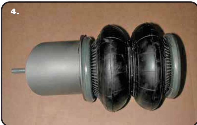
4. Assemble the upper cup bracket to the air spring, using 3/8"-16 Nylok nuts and 3/8" flat washers. Torque the 3/8" nuts 15-20 ft-lbs.
