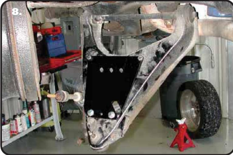
**8.** Bolt the lower air spring plate to the lower arm. The two outer holes will align with the factory bump stop holes. The inner two holes must be drilled. Use the bumpstop to bolt the outer part of the plate to the control arm. Use a 3/8" drill bit to drill the inner 2 holes. Install a 3/8" flat washer on each of (2) 3/8"-16 bolts and insert them into the holes. Install a 3/8" flat washer and 3/8"-16 nylok nut on the threads of the bolt. Torque to 30 ft-lbs.
