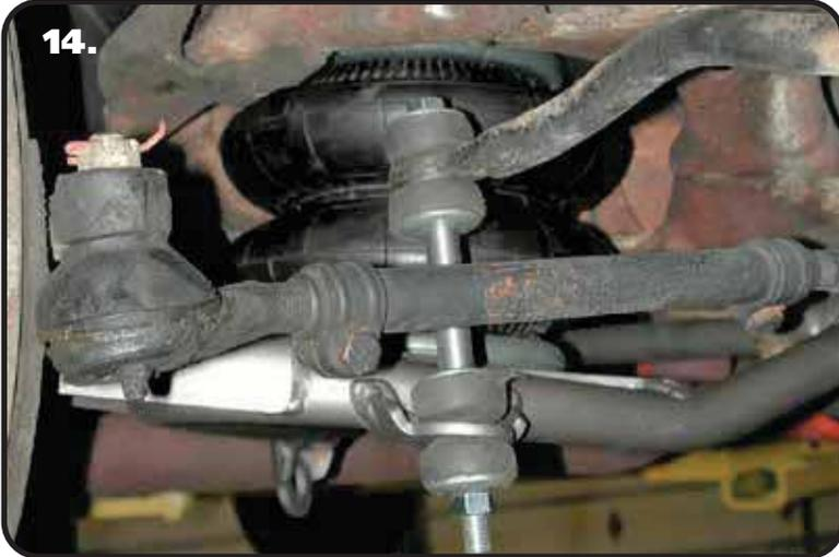
**14.** To correct the sway bar alignment the end link must be shortened to 2" tall. A 3/8"-16 x 6 1/2" bolt is supplied.
