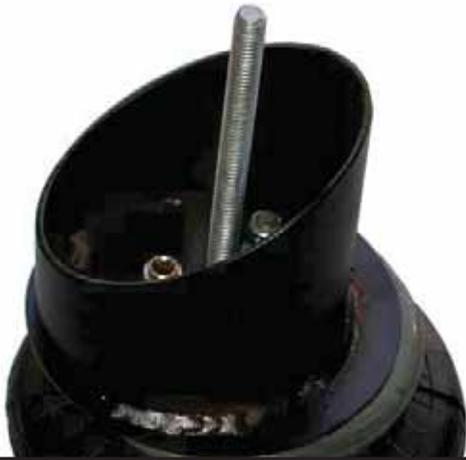
5. Thread the 8" stud into the nut in the bottom of the cup.
