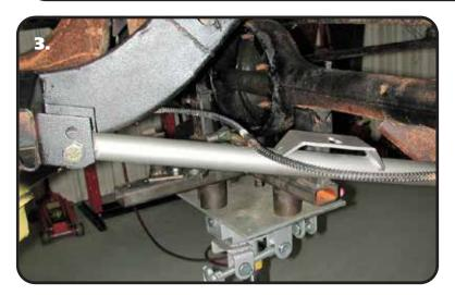
**3.** Fasten the front of the lower StrongArms to the frame using the 5/8" x 3 ¾" bolts, flat washers, and nylok nuts supplied. The OEM rear bolt will be reused in conjunction with the supplied flat washer and Nylok nut. Tighten the bolts/nuts enough to eliminate any gaps.
