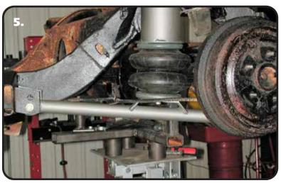
**5.** Thread the  $3/8"-16 \times 3/4"$  bolt with washer and lock washer about half way into the air spring. Slide bolt into slot on lower arm and tighten 15-20 ft-lbs.
