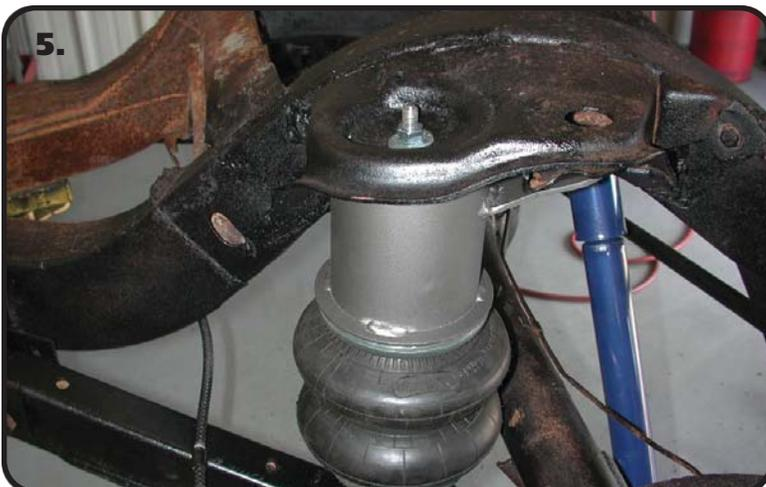
5. Place the air spring assembly into the coil spring pocket with the tab on the side of the cup aligning with the factory bump stop mount. The stud should poke through the hole in the upper coil spring pocket. Some cars may not have this hole and it must be drilled with a 7/16" drill bit. Fasten with a 7/16" Nylok nut and flat washer. Torque 25-35 ft-lbs.
