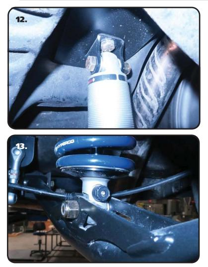
**12.** Insert the shock bearing t-bushings into the bearing of the shock body. Insert the shock into the upper mount, lining up the holes of the mount and shock. Install a 1/2" flat washer on a  $1/2"-13 \times 2 \ 1/2"$  bolt. Insert the bolt/washer into the upper mount/shock. Install a 1/2" flat washer and 1/2"-13 nylok nut and Torque to 50 ftlbs.
