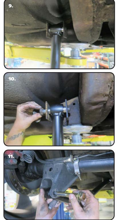
**9.** The Lower Control Arm has the bottom CoilOver mount built in, it will need to be installed with the CoilOver mount up and to the rear of the car. Install a 5/8" ID R-joint Spacer into the front R-joint. The Small Diameter goes into the R-joint. Slide the R-joint into the OEM lower control arm mount. Align the holes in the frame with the thru-hole of the R-Joint.
