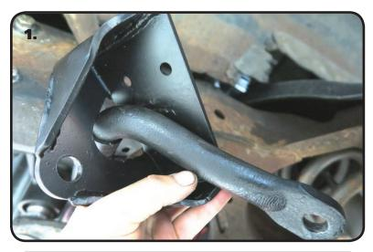
**1.** With the swaybar in position, slide the Slave Cylinder bracket over the end of the swaybar with the mounting holes to the OUTSIDE of the car. Position the bracket in the area it will be mounted.
