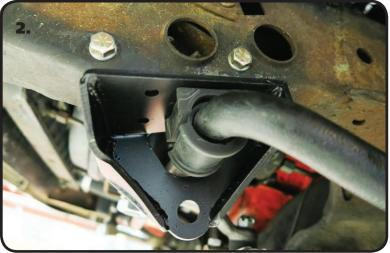
**2.** Open up the Poly SwayBar Bushings and install them over the Delrin Sleeves.
