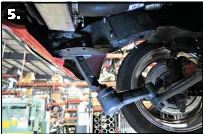
5. Disconnect the idler arms from the frame.
