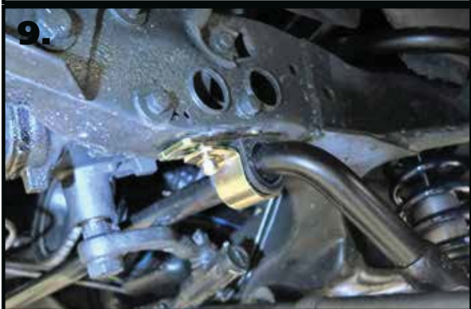
9. Lift the bar in position, the bolts sticking through the frame and spacer will go in the slots of the bushing strap. Hold the bar in place & install a 5/16" flat washer and 5/16"-18 nylok nut on the threads of each bolt sticking through the slots of the bushing strap. Repeat steps 8-10 on the opposite side, but do not tighten the hardware at this time.
