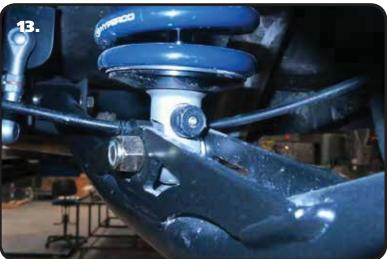
**13.** Insert the shock bearing t-bushings into the bearing of the shock eyelet. Insert the shock into the lower control arm, lining up the holes of the mount and shock. Install a 1/2" flat washer on a 1/2"-13 x 2 1/2" bolt. Insert the bolt/washer into the upper mount/ shock. Install a 1/2" flat washer and 1/2"-13 nylok nut and Torque to 50 ftlbs.
