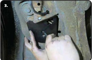
**3.** The upper mount bolts into the car and will require the holes to be drilled. Start by holding the plate up in the car aligning the back edge with the body mount. Mark the holes on the frame.
