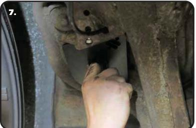
**7.** Position the Shock Mount/Plate up into the frame, holding the shock mount and hardware in place.
