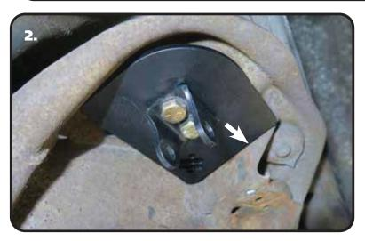
2. This kit contains a Upper Shock Mount setup that will require drilling to install it. Image 2 is of the upper mount installed, we will cover the installation in the next steps. The rear of the plate will need to be aligned with the body mount that is to the rear of the coil spring mount. See the ARROW in Image 2.
