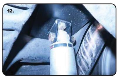
**12.** Insert the shock bearing t-bushings into the bearing of the shock body. Insert the shock into the upper mount, lining up the holes of the mount and shock. Install a 1/2" flat washer on a 1/2"-13 x 2 1/2" bolt. Insert the bolt/washer into the upper mount/shock. Install a 1/2" flat washer and 1/2"-13 nylok nut and Torque to 50 ftlbs.
