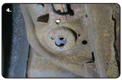
**4.** The frames of these cars varied through the years, some have a center hole, some are solid. The frame we are doing this install on has a center hole. If the frame is solid, drill the marked holes with a 1/2" drill bit. Frames with the center hole will require a die-grinder or something similar to notch the edges of the center hole. We used a die-grinder with a burr bit to notch the holes. Repeat **Steps 2-4** on the opposite side.
