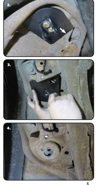
2. This kit contains a Upper Shock Mount setup that will require drilling to install it. Image 2 is of the upper mount installed, we will cover the installation in the next steps. The rear of the plate will need to be aligned with the body mount that is to the rear of the coil spring mount. See the ARROW in Image 2.
