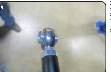
**3.** Install the <sup>3</sup>/<sub>4</sub>" jam nut onto the end of the Heim end, then screw Heim end into the end of the panhard bar. Set the Panhard Bar to 31.500". You may need to readjust it after getting the car set at ride height, but this is a good starting point. Press the SMALL diameter of the aluminum 9/16" ID T-bushings into the Heim end.
