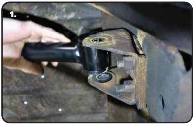
**1.** Insert the Bushing end of the Upper Control Arm into the OEM mount. The control arm should be installed with the bend upward for better axle clearance. Install a 5/8" flat washer on a  $5/8"-18 \times 3 3/4"$  hex bolt through the mount and control arm bushing. Install a 5/8" flat washer, followed by a 5/8"-18 nylok jam nut onto the threads of the bolt. Tighten the hardware enough to eliminate any gaps.
