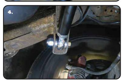
**4.** Insert the heim end of the panhard bar into the OEM frame mount. Align the align hole in the heim end with the holes in the OEM mount. Install a 9/16" flat washer on a 9/16"-18 x 2 3/4" hex bolt and insert in into the aligned holes. Install a 2nd 9/16" washer followed by a 9/16"-18 nylok nut on the threads of the bolt sticking through the frame. Torque to 95 ftlbs.
