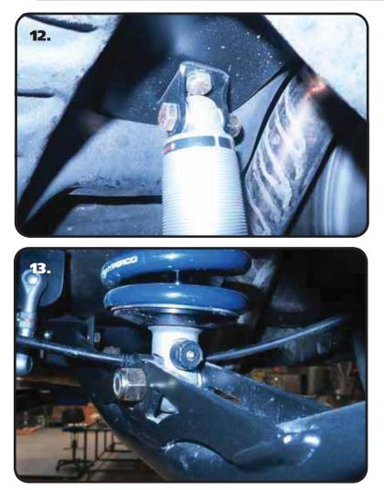
**12.** Insert the shock bearing t-bushings into the bearing of the shock body. Insert the shock into the upper mount, lining up the holes of the mount and shock. Install a 1/2" flat washer on a  $1/2"-13 \times 2 \times 1/2"$  bolt. Insert the bolt/washer into the upper mount/shock. Install a 1/2" flat washer and 1/2"-13 nylok nut and Torque to 50 ftlbs.
