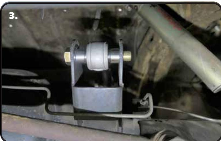
**3.** Install a 5/8" flat washer on a 5/8"-18 x 3 3/4" hex bolt through the mount and control arm R-Joint. Install a 5/8" flat washer, followed by a 5/8"-18 nylok jam nut onto the threads of the bolt. Tighten the hardware enough to eliminate any gaps.
