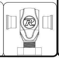
New R-Joints will be quite stiff (75-90 in/lbs breakaway torque) until they "break in" after a few miles of use. After the break in period they will move much more freely. Because the composite bearing race contains self lubricating ingredients, no additional lubrication is needed or desired. Any additional lubrication will only serve to attract more dirt and debris to the R-Joint and actually shorten its life.
