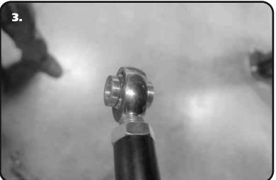
**3.** Press the SMALL diameter of the aluminum 9/16" ID T-bushings into the Heim end.
