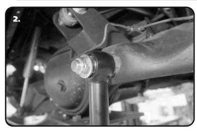
**2.** Install a Narrow 5/8" ID R-joint Spacer into the R-joint. The Small Diameter goes into the R-joint. Slide the R-joint onto the stud and fasten in place with a 5/8" flat washer and 5/8"-18 thin jam nylok nut. Torque to 95 ftlbs.
