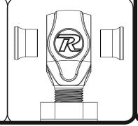
New R-Joints will be quite stiff (75-90 in/lbs breakaway torque) until they "break in" after a few miles of use. After the break in period they will move much more freely. Because the composite bearing race contains self lubricating ingredients, no additional lubrication is needed or desired. Any additional lubrication will only serve to attract more dirt and debris to the R-Joint and actually shorten its life.
