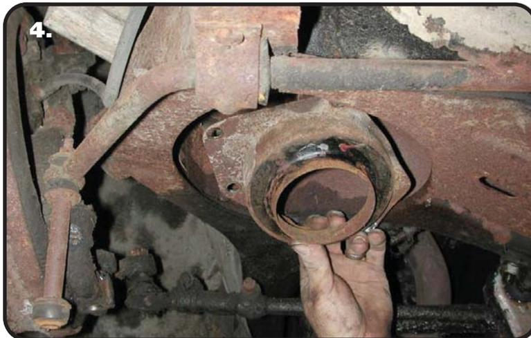
4. The upper coil spring retainer needs to be taken out as well. It is secured with rivets that need to be ground down or drilled out from the top. Some cars may have bolts instead of rivets. Also remove the Shock Bushing Cup and drill the Shock Hole to 3/4". A Unibit works well for this.
