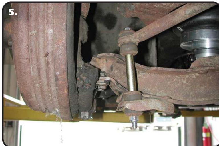
5. For better sway bar alignment the end link must be cut down by 1" to 2 1/2" long. 3/8" x 6 1/2" Hex Bolts and 3/8" Nylok Nuts are included in the kit to replace the OEM hardware after shortening the sway bar end link.
