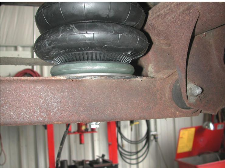
6. Use the 3/8" x 3 1/2" bolt and lower plate to secure bag to the lower arm.
