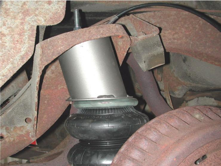
4. Install airline fitting into airspring using thread sealant. The airline will also need to be routed at this time. Bolt the upper cup bracket to the top of the airspring using the two 3/8" nyloc nuts supplied.
