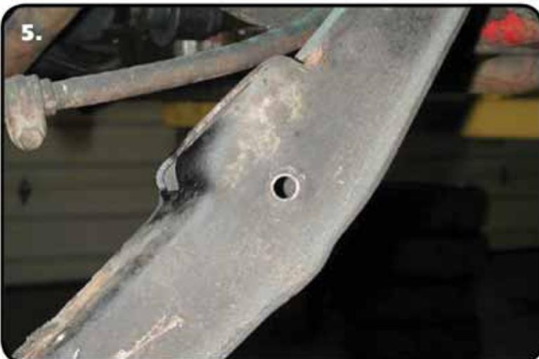
5. The lower shock mount hole will be used to mount the Shockwave. This hole must be drilled out to 1/2".
