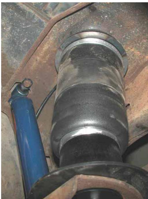
4. Apply thread sealant an elbow air fitting and screw it into the top of air spring.
