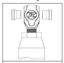
Insert the SMALL end of the spacer INTO each side of the center pivot ball. Push the spacer in until it bottoms out in the center pivot.
