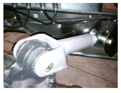
4. Fasten the other end of the bar to the axle using a ½" x 3 ½" bolt and Nylok nut.
