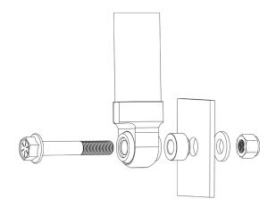
2. The shock must be relocated to the front side of the control arm. A .625" hole must be drilled in the lower control arm for the Cantilever pin to attach. This hole will be drill directly in front of the factory shock mount but may need to be moved in or out slightly to allow for maximum tire clearance and turning radius.
