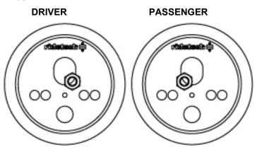
**NOTE:** THIS KIT HAS A DRIVER AND PASSENGER UPPER CUP BRACKET. A TOP VIEW IS SHOWN ABOVE.
