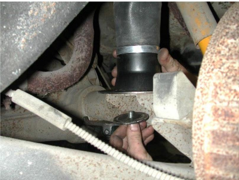
6. Hold the air spring assembly up to the coil spring pocket with the stud protruding through the hole in the center of the coil spring pocket. Place the 4" diameter washer over the stud and tighten with a 7/16" Nyloc nut and flat washer.
