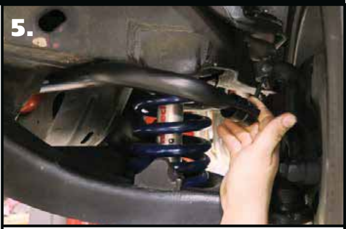
5. Insert the sway bar in the stock location. See below for installation tips.
