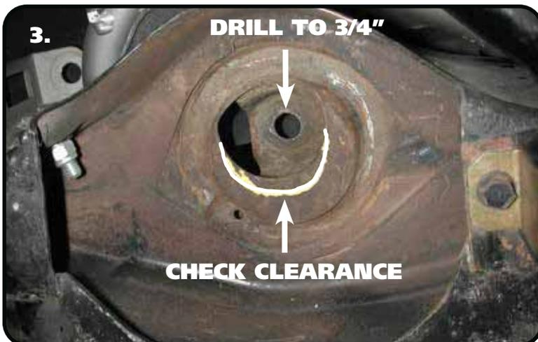
3. Drill the OEM shock hole out to 3/4". This can be done with a Unibit. The CoilOver stud top will come in contact with the coil spring retainer, so it must be opened up towards the engine. A die grinder works well here.
