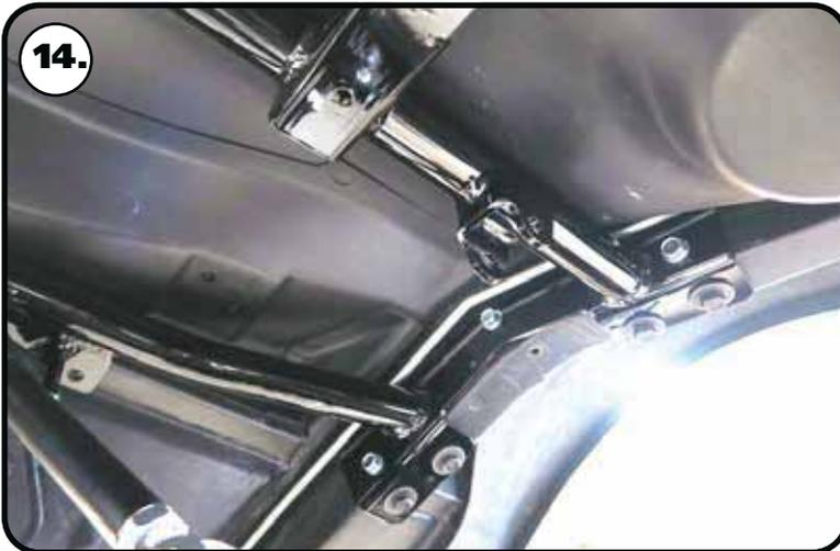
**14.** Install a 3/8" split lock washer & 3/8" flat washer on each of the 3/8"-16 x 1 1/4" bolts supplied in the kit. Thread them into the riv-nuts. Torque to 23 ft-lbs. Torque the front tab and sway bar tab hardware to 30 ft-lbs.
