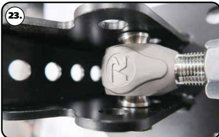
**23. Image 23** shows a bottom view of the bar installed. Notice the spacers in each side of the R-Joint.
