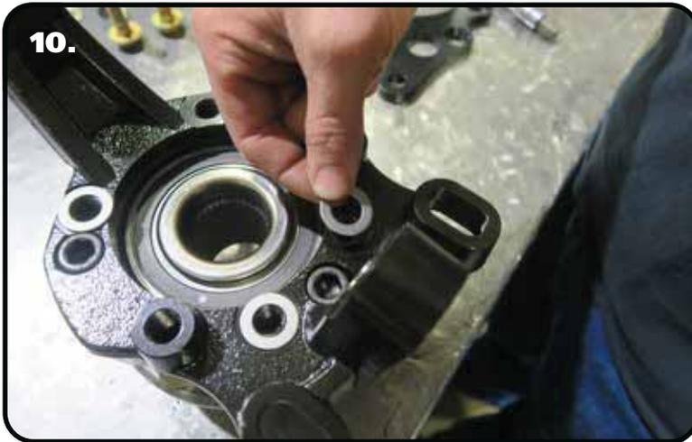
**10.** Lay a .062" thick, 1/2" ID shim on each of the caliper brackets (3) mounting holes.
