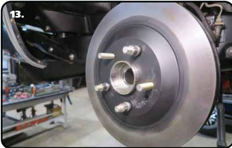
**13.** Install the rotor on the hub. Thread some lug nuts on the threads of the hub to hold the rotor tight on the hub.
