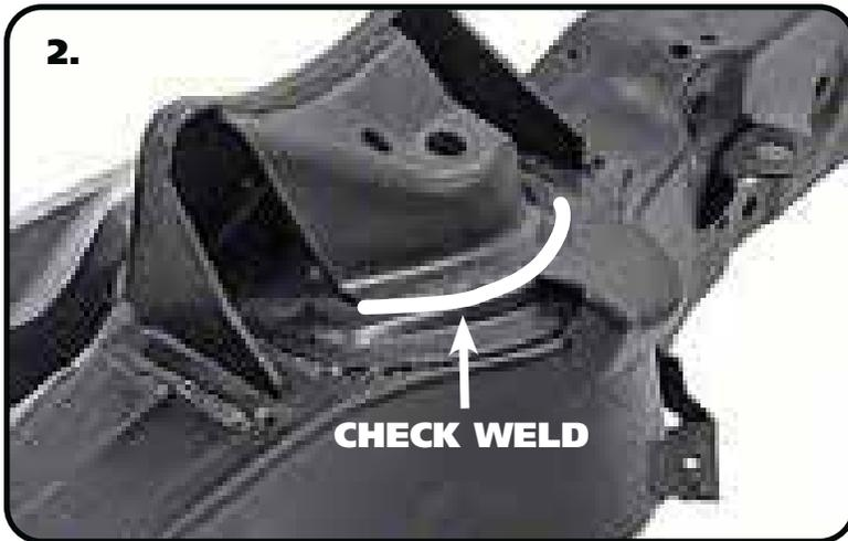
2. Check the weld in the area pointed out. We have seen some very poor factory welds in this area. If it doesn't look adequate to support the vehicle, reweld the area.
