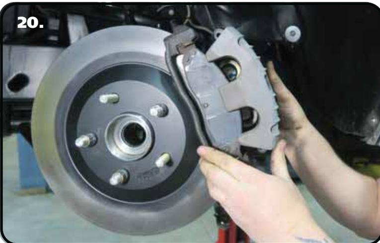
**20.** Install the brake pads and caliper.
