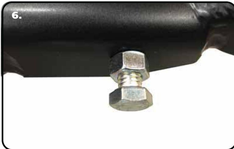
6. Thread the 3/8"-16 nut onto the 3/8"-16 x 1 1/4" bolt. Thread it into the front hole of the ball joint plate. You will need to adjust the steering stop to suite your needs. This setting will vary depending on wheel and tire size and other suspension components. Torque to 12 ft-lbs.
