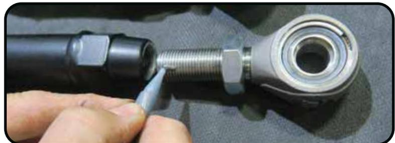
**14d.** Thread the r-joints into the 4-link bar. Thread them in evenly until you achieve the correct center to center length.
