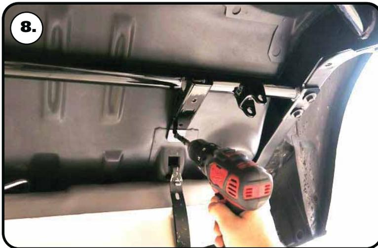
**8.** Drill a 3/8" hole through the each of the sway bar mount tabs. These holes will go into the trunk so make sure nothing is in the trunk floor. If there is a mat, remove it before drilling the holes.
