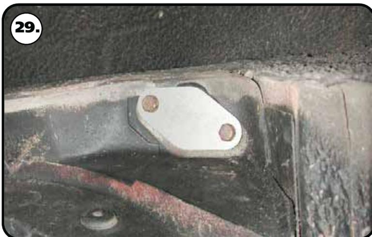
**29.** Bolt the Shock Block Off Plates in place of the OEM upper shock mounts using the OEM hardware. If you are running Mini Tubs, these mounts do not exist any more.
