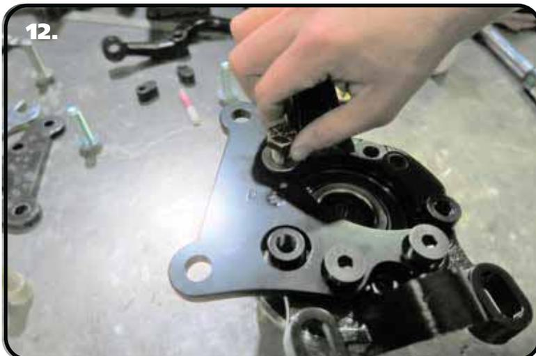
**12.** Insert a 1/2"-13 x 1 1/4" flat head socket cap screw in each of the lower mounting holes. Install a 1/2" flat washer on a 1/2"-13 x 1 1/4" hex bolt and insert it in the upper mounting hole. Tighten the hardware to 75 ft-lbs.
