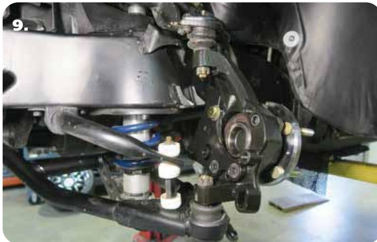
**9.** Attach the spindles to the control arms. Torque the ball joints using the torque specs below.
