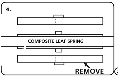
**4.** The original StreetGrip kit came with a clamping plate on the top and bottom of the composite leaf spring. The BOTTOM plates will need to be removed.
