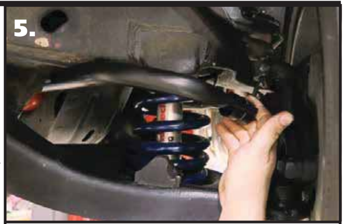
5. Insert the sway bar in the stock location. See below for installation tips.
