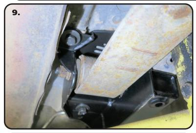
**9.** Position the rear of the subframe connector so that the mounting holes line up with the u-nuts in the OEM locations. Install (2) 3/8"-16 x 1 1/2" conical bolts in the outer 2 holes of the subframe connector. Leave the hardware loose until later.
