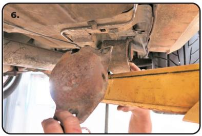
**6.** Remove the OEM leaf spring mount from the front of the leaf spring. Retain the leaf spring hardware for reassembly. Replace the OEM U-nuts in the floor pan and frame rail with the new ones supplied in the hardware kit.
