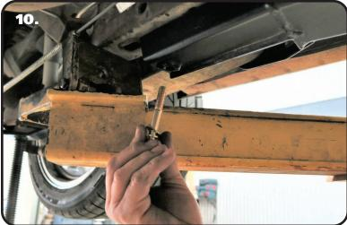
**10.** Install a 3/8" flat washer on a 3/8"-16 x 2 1/2" hex bolt. Insert the bolt/washer in the inner hole of the subframe connector. This hole goes through the tube of the subframe connector and lines up with the u-nut that is in the OEM frame rail. Thread the bolt into the u-nut. Leave the hardware loose until later.
