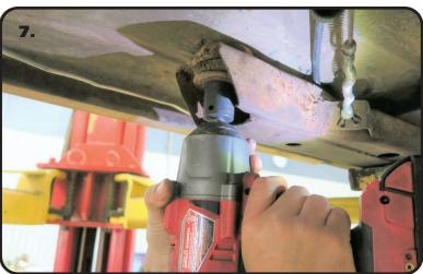
**7.** Remove the REAR body bushing bolt from the front subframe. Retain the body bushing bolt and bottom half of the body bushing for reassembly.
