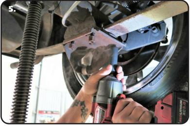
**5.** Remove the leaf spring lower clamp plate. Retain the Hardware for reinstallation.
