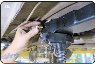
**13.** Install a 5/16" flat washer on each of (4) 5/16"-18 x 1" bolts. Insert a bolt/washer in each of the 4 holes. Install a 5/16" flat washer and 5/16"-18 nylok nut on the threads of each of the (4) bolts. Torque the hardware to 25 ftlbs.
