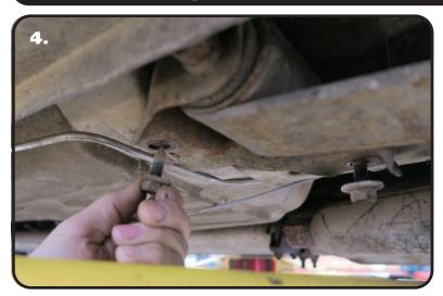
**4.** Support the center of the differential with a jack. Remove the 3 bolts from the OEM leaf spring mounts. Do this for both sides.
