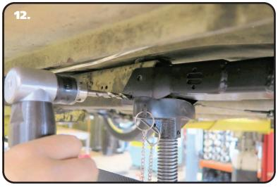
12. The 4 mounting holes in the front of the subframe connector will be used as a template to drill the new holes in the OEM subframe. IF YOU ARE USING RUBBER BUSHINGS, YOU WILL NEED TO JACK THE FRONT OF THE SUBFRAME CONNECTOR UP TIGHT AGAINST THE OEM SUBFRAME. Solid body bushings will hold the subframe connector tight against the OEM subframe. Tighten the (3) REAR subframe mounting bolts that were left loose in steps 9 and 10 to 30 ftlbs. Drill the 4 holes with a 5/16" drill bit.
