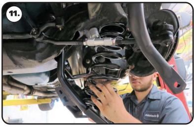
**11.** Reinstall the coil spring, making sure the end of the coil spring is nested in the provision in the frame. Rotate the coil spring isolator to align it with the bottom of the coil spring.
