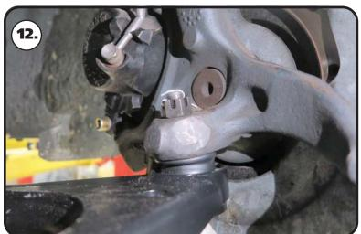
**12.** Attach the spindle to the control arms.
