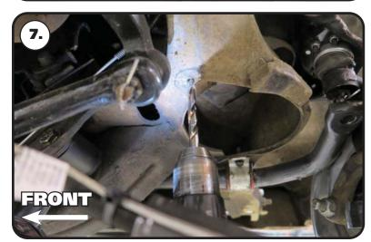
**7.** Use a 3/8" drill bit to drill a hole at the center of the bump stop spacer location.
