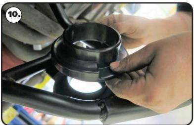
10. The kit includes 2 different size coil spring isolators. Verify which size fits your coil spring the best. Place the coil spring isolator over the ring of the control arm.
