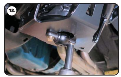
**13.** Reinstall the shocks using the supplied 5/16" hardware to attach them to the new control arms. Torque to 17 ft-lbs.
