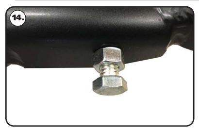
**14.** Thread the 5/16''-18 nut onto the  $5/8''-18 \times 1 \frac{1}{4}''$  bolt. Thread it into the rear hole of the ball joint plate. You will need to adjust the steering stop to suite your needs. This setting will vary depending on wheel and tire size and other suspension components.
