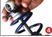
Once the knob is removed slide a Delrin washer over the eyelet. Next, slide the upper spring mount (803-00-199) over eyelet as seen in figure 4.
