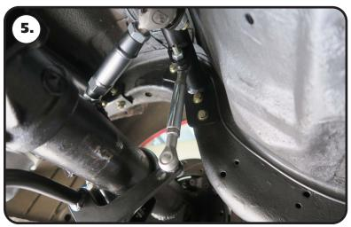
**5.** Attach the bottom of the PosiLink to the front hole of the sway bar arm. We recommend starting in the front hole. Install a 3/8" flat washer and M10-1.5 nylok nut. Install the 2nd PosiLink in the other sway bar arm and torque the nuts to 37 ft-lbs.
