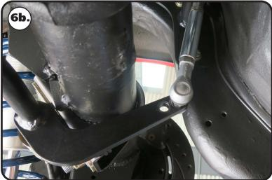
**6b. Image 6b** shows the sway bar arm position in relationship to the axle. The shocks will not allow the rear differential to droop any lower than this position. You need just enough clearance on the axle tube to keep it from hitting. Torque the u-bolt hardware to 55 ft-lbs.
