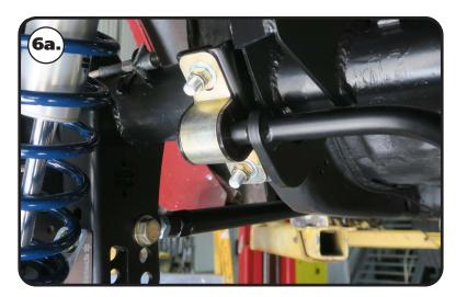
6a & 6b. For this step, the axle needs to hanging at full droop on the ShockWaves/CoilOvers. Rotate the sway bar mounts rearward until the sway bar arms just clear the bottom of the axle.
