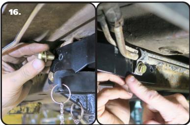
**16.** Install a 5/16" flat washer on each of (4) 5/16"-18 x 1" bolts. Insert a bolt/washer in each of the 4 holes. Install the brake/fuel line clamp using the rear hole of the passenger subframe connector. Install a 5/16" flat washer and 5/16"-18 nylok nut on the threads of each of the (4) bolts. Torque the hardware to 25 ftlbs.
