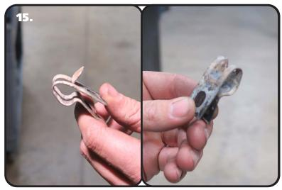
**15.** If your brake/fuel line clamp has a tab sticking out of the rear, it will need to be flattened or cut off.
