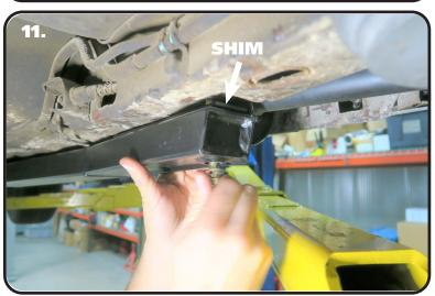
11. Install a 3/8" split lock washer and 3/8" flat washer on a 3/8"-16 x 3" hex bolt. Insert the bolt/washer in the inner hole of the subframe connector. This hole goes through the tube of the subframe connector and lines up with the u-nut that is in the OEM frame rail. Thread the bolt into the u-nut. Leave the hardware loose until later.
