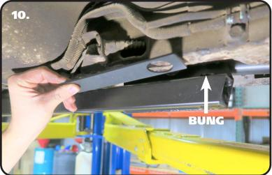
**10.** Place the shim on top of the subframe connector tube with the hole in the shim over the rear bung.
