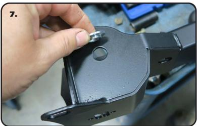
7. The kit includes a Driver and Passenger subframe connector. The leaf spring mount is positioned to the outside of the car with the subframe connector tube dipping down to clear the floor pan. The leaf spring mounting holes in the subframe connector's are 5/8" for many aftermarket suspensions. The kit includes T-bushings for using 1/2" hardware. If you are using 1/2" hardware, insert a t-bushing in each leaf spring mounting hole. The large OD will be on the outside of the leaf spring pocket.
