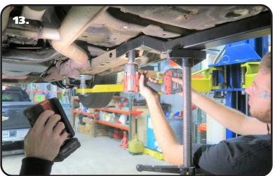
13. IF YOU ARE USING RUBBER BUSHINGS, YOU WILL NEED TO JACK THE FRONT OF THE SUBFRAME CONNECTOR UP TIGHT AGAINST THE OEM SUBFRAME. Solid body bushings will hold the subframe connector tight against the OEM subframe. Tighten the (3) REAR subframe mounting bolts that were left loose in **Steps 9** - **11** to 30 ftlbs. We use a stand to push the front of the connector up tight against the frame rail. Tighten the OEM body bushing bolt.
