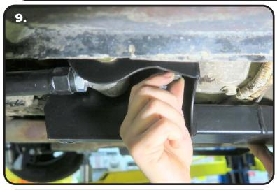
**9.** Position the rear of the subframe connector so that the mounting holes line up with the u-nuts in the OEM locations. Start (2) 3/8"-16 x 1 1/2" conical bolts in the outer 2 holes of the subframe connector. This hardware needs to need left loose enough to insert the shim in the next step.
