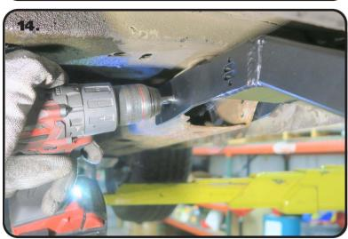
**14.** The 4 mounting holes in the front of the subframe connector will be used as a template to drill the new holes in the OEM subframe. Drill the 4 holes with a 5/16" drill bit.
