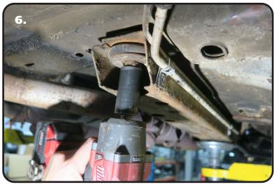
**6.** Remove the REAR body bushing bolt from the front subframe. Retain the body bushing bolt and bottom half of the body bushing for reassembly. Unbolt the brake/fuel line clamp from the rear of passenger the subframe rail.
