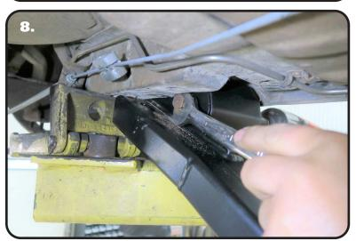
**8.** Attach the rear of the subframe connector to the front of the leaf spring. Install the leaf spring bolt from the outside of the car with the nut to the inside. The leaf spring bolt will need to be tightened before the subframe connector is installed.
