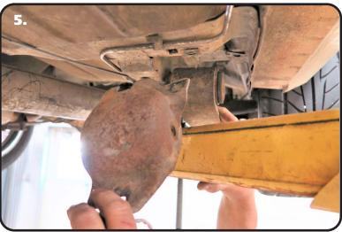
**5.** Remove the OEM leaf spring mount from the front of the leaf spring. Retain the leaf spring hardware for reassembly. Replace the OEM U-nuts in the floor pan and frame rail with the new ones supplied in the hardware kit.
