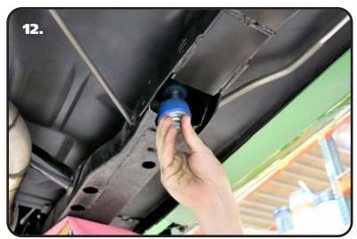
**12.** Push the front subframe connectors up against the OEM subframe. Reinstall the OEM body bushing/bolt.
