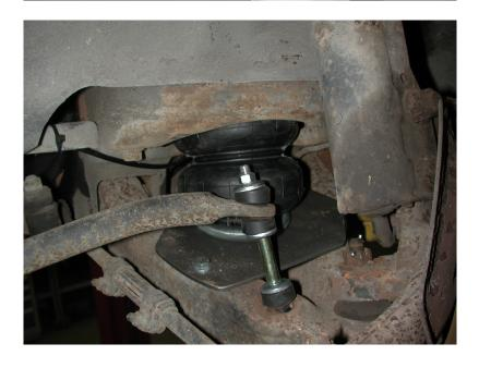
6. Set the air spring plate on the lower control arm. The plate will index off of the factory bump stop hole. Insert a 3/8" x 1 1/4" with Nylok and flat washers.
