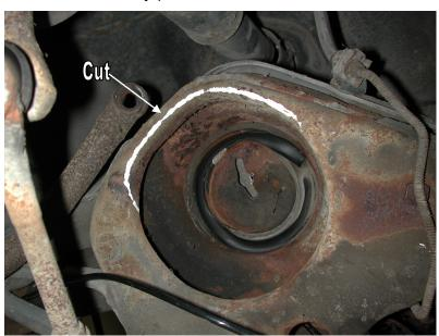
3. The outer lip of the coil spring pocket must be removed for air spring clearance. This is best done with a cut off wheel or plasma cutter. Grind smooth when finished.
