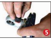
Install upper spring mount retainer clip (803-00-199) into the groove on the upper eyelet as seen in figure 5. Then, reinstall adjuster to complete assembly.
