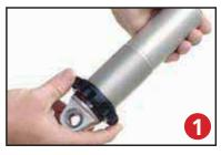
First, using the supplied lower adjuster nut (803-00-199) thread the nut onto the shock from the bottom side as seen in figure 1. Remove the plastic pellet that is in the split of the adjuster nut.
