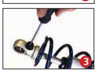
Before the upper spring mount can be installed screw the adjuster knob on the upper eye mount to the firmest setting (clockwise) as seen in figure 3. Then remove the Knob by holding it while removing the center screw.
