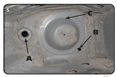
**5.** Picture "5" shows the factory upper coilspring pocket in the car. (A) is the factory shock hole that the upper plate and mounting bracket will be bolted through, (B) is a locating hole in the body that will be used to help locate the new upper plate, (C) is the factory coilpring locator that will also help in locating the upper plate
