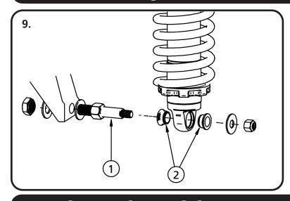
**9.** Drill the factory shock stud hole out to 5/8", this can be done using a Unibit. Install the (1) Shock stud (90001617) into the factory lower mount using the hardware supplied with the stud. Install a 5/8" I.D. spacer on the shock stud, then the bottom of the ShockWave on the stud, followed be another 5/8" I.D. spacer. Install 7/16" washer and Nylok nut.
