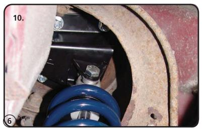
sure that the locking screw is lightly tightened in the adjuster nut. Once you have preloaded tighten the locking screw. It may be necessary to add more preload, this will be determined once the car is setting on the ground.
