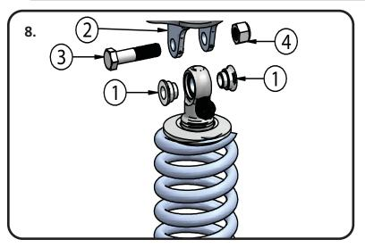
**8.** With the CoilOver assembled insert the upper spacers(1) into the upper shock bearings. With the spacers installed insert the CoilOver assembly into the upper shock mount(2). Align the holes in the bracket with the hole in the Shock spacers and insert the 1/2" Bolt(3) and secure with the 1/2" Nylok Nut(4).
