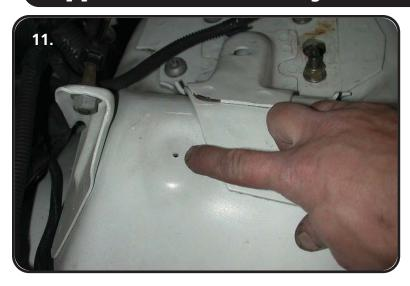
11. A bump stop will be installed between the inner fender and upper control arm to ensure that the tire does not hit the inner fender when fully compressed. There is a small hole on the inner fender that must be drilled out to 3/8". Fasten the bump stop to the inner fender using a 3/8" Nylok nut and flat washer.
