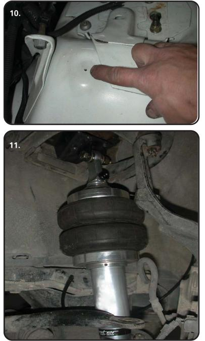
**10.** A bump stop will be installed between the inner fender and upper control arm to ensure that the tire does not hit the inner fender when fully compressed. There is a small hole on the inner fender that must be drilled out to 3/8". Fasten the bump stop to the inner fender using a 3/8" Nylok nut and flat washer.
